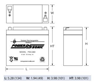
Tolerances are +/- 0.04 in. (+/- 1mm) and +/- 0.08 in. (+/- 2mm) for height dimensions. All data subject to change without notice.
